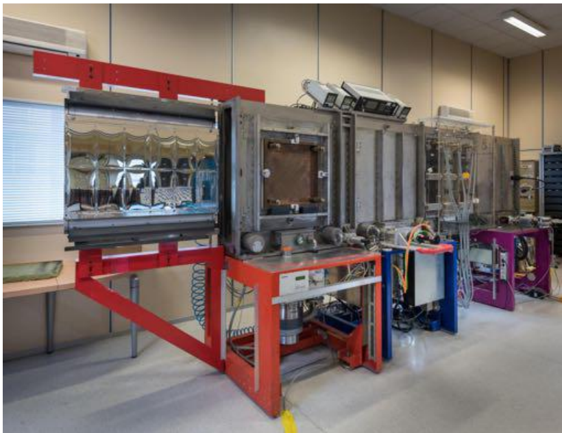
Sputtering machine PI Production 0.8 m 2 / jour
