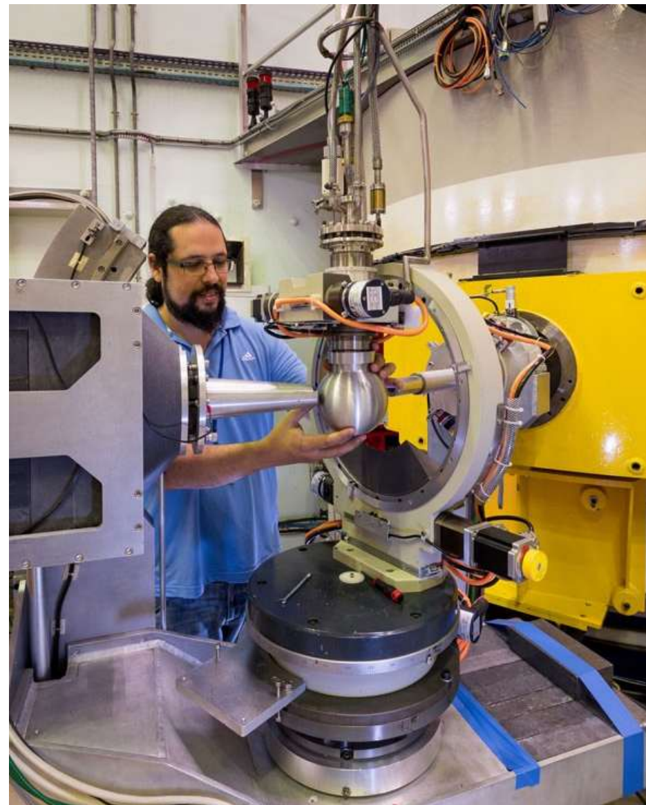
Hot neutron 4-circle diffractometer D9 @ ILL
