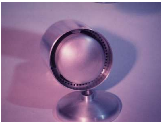
Lenticular to annular in 1995 Ø ext =130mm Ø int =110mm h=300mm T=20K 400mm from core
